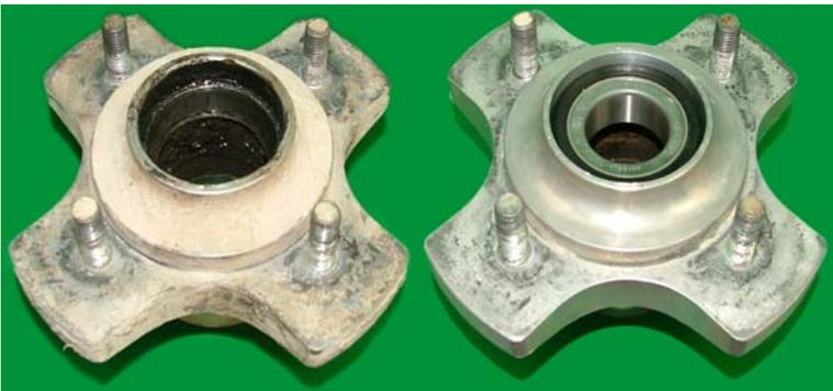
When faced with the problem we suggested manufacturing a new thicker stud that could be welded to the existing assembly. This new stud would not only be able to withstand more force than the original, but also cost less and was available on a shorter lead time. We were also able to machine and fit new quality bearings in the wheel hub, this again increased the overall strength of the assembly.
